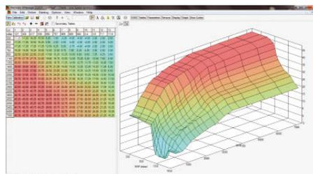
A Low cam Fuel table on S300 showing load which is this time a Throttle Position Sensor % value vs RPM. This type of calibration table is described as AlphaN.
