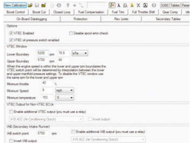
Note that there is also an activation temperature setting which means you can't push the engine hard until it's fully warmed up.
